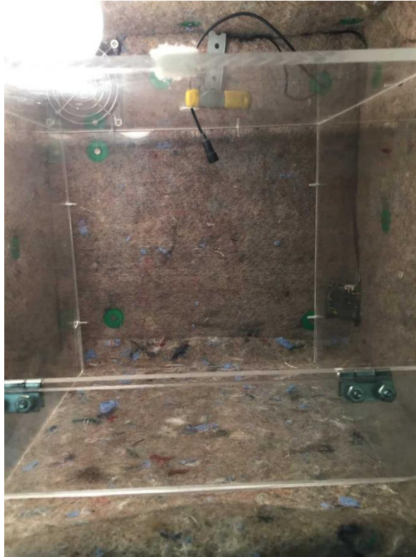
Figure 4. Plexiglas chamber. Surrounded by sound attenuating media with a microphone inserted inside to record separation-induced vocalizations aimed at modeling anxiety and depression.
