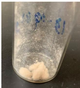
**Figure 36.** The crystalline solid obtained from the reaction of propane-1,3-bis(aminophenol) (**3a**) and benzene diboronic acid (**7**).
