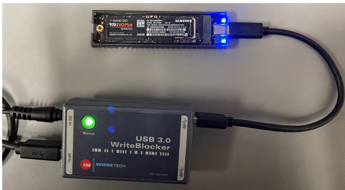
Fig. 7.1. Samsung NVMe SSD attached with USB WriteBlocker.
