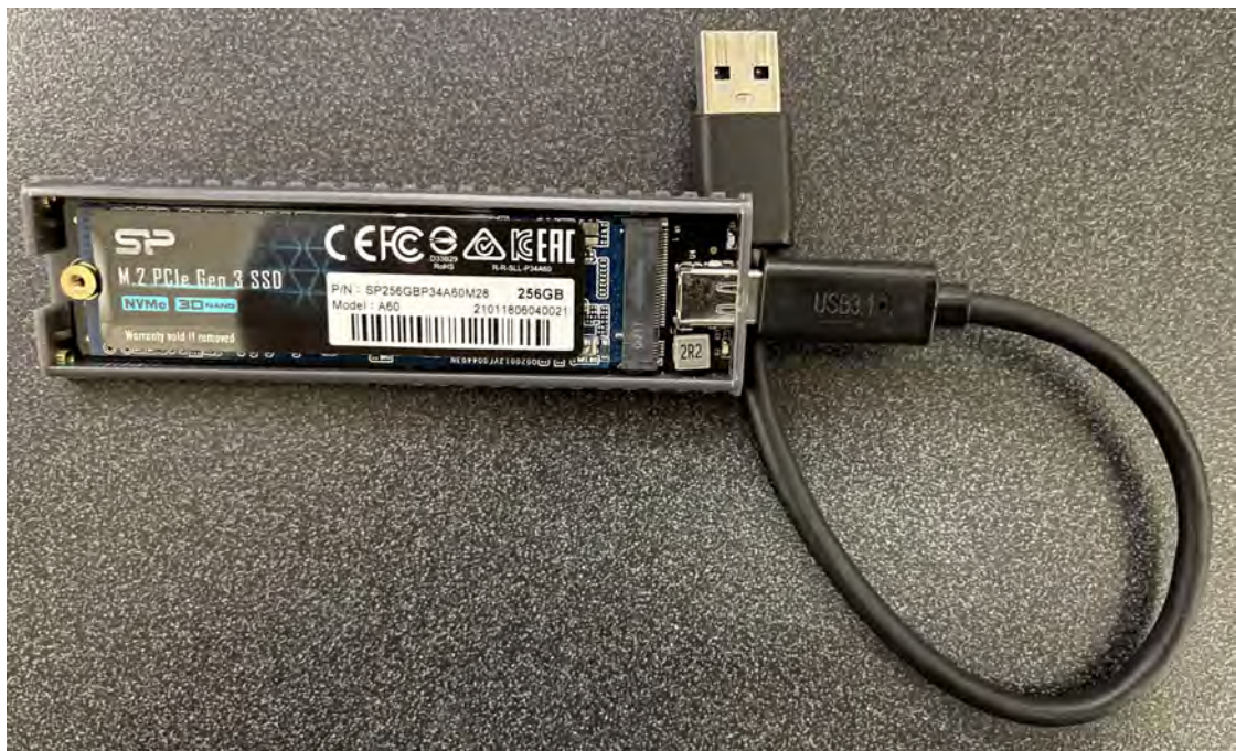
Fig. 8.4. Silicon Power NVMe SSD attached without USB WriteBlocker.
