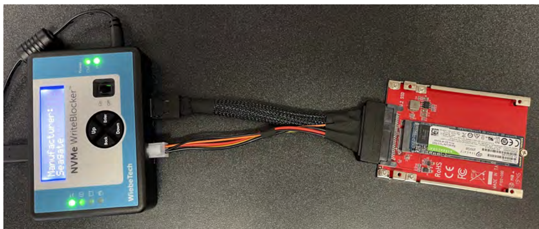
Fig. 9.2. Seagate NVMe SSD attached with NVMe WriteBlocker.
