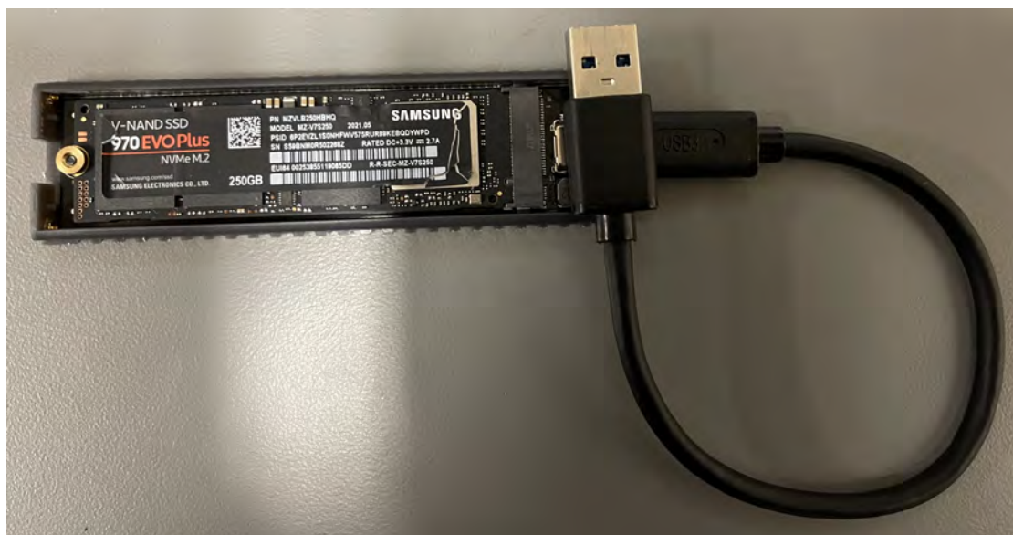
Fig. 8.1. Samsung NVMe SSD attached without USB WriteBlocker.
