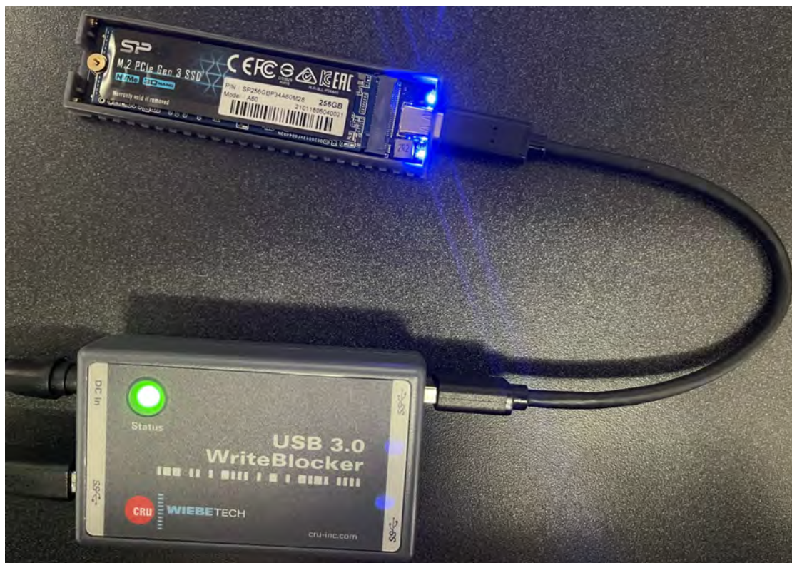
Fig. 7.4. Silicon Power NVMe SSD attached with USB WriteBlocker.
