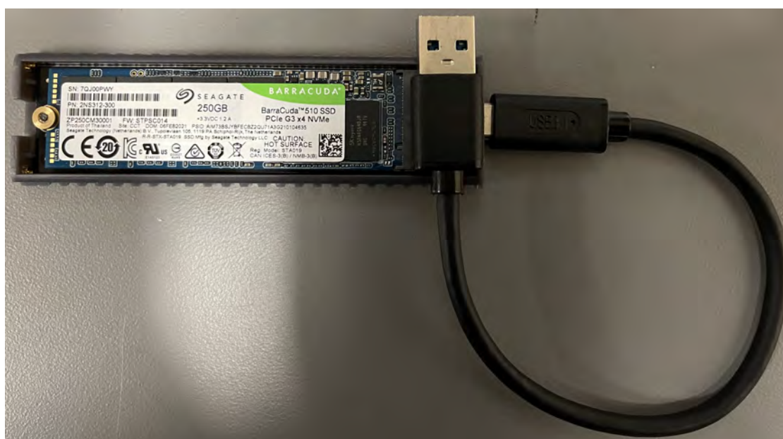
Fig. 8.2. Seagate NVMe SSD attached without USB WriteBlocker.
