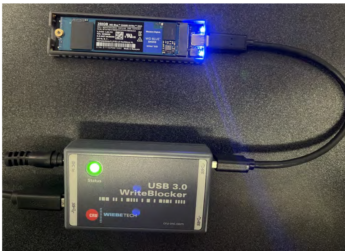
Fig. 7.3. Western Digital NVMe SSD attached with USB WriteBlocker.
