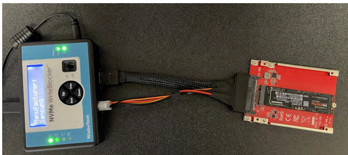
Fig. 9.1. Samsung NVMe SSD attached with NVMe WriteBlocker.
