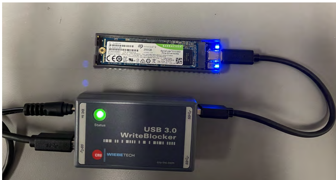
Fig. 7.2. Seagate NVMe SSD attached with USB WriteBlocker.
