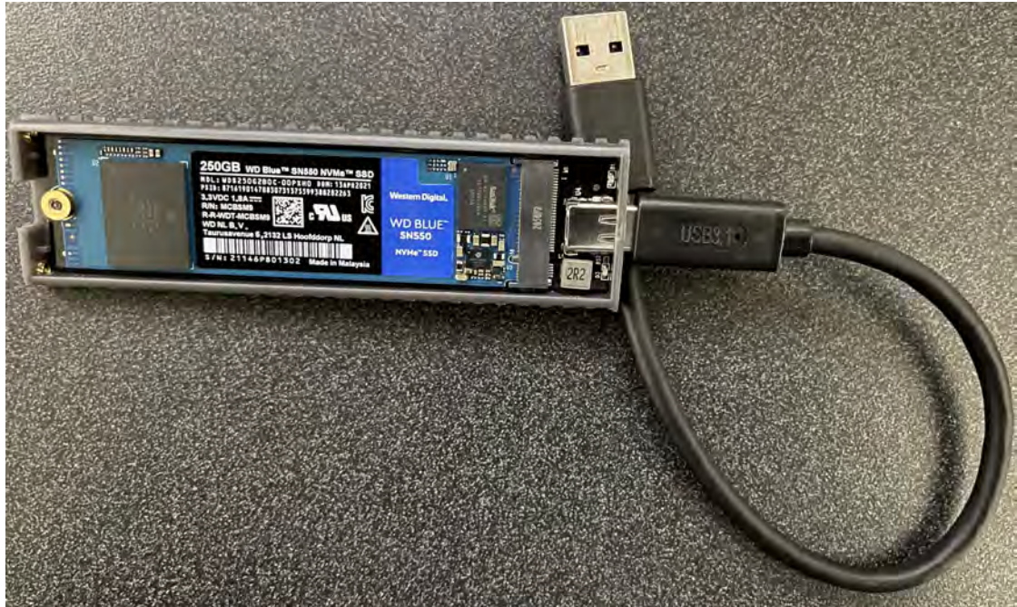
Fig. 8.3. Western Digital NVMe SSD attached without USB WriteBlocker.
