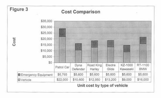
Analysis associated with maintenance and gasoline consumption show that a motorcycle is more cost efficient to operate than a patrol car. Average maintenance per mile driven for a motorcycle is \$0.0742 per mile driven compared to a patrol car at \$0.081 (Streff, 1994).
