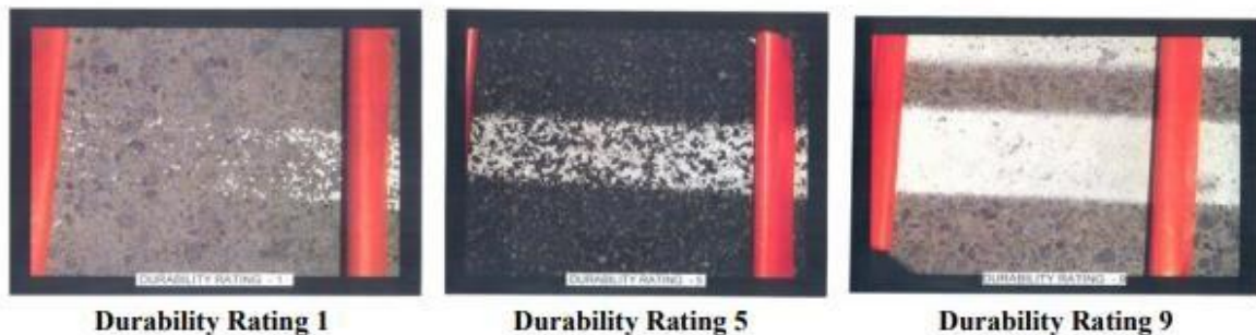
Figure 2. Durability Rating of 1 (Left) and Durability Rating of 9 (Right)
