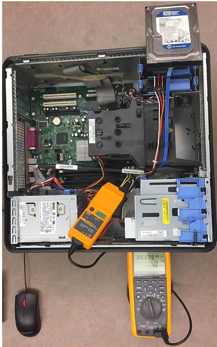
Fig. 1. Collection environment for power analysis.
